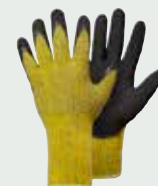
987 Nitrile, 7 gg, palm-dipped, long cuff, Para-aramid, contact heat < 250°C p.124
